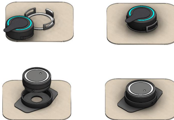
Figure 4: Different approaches considered to put off the enclosure in the patch.
