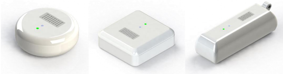
Figure 3: Prototypes of the enclosure, presenting various shapes for comparison. Left: circular shape; centre: square shape; right: rectangular shape.
